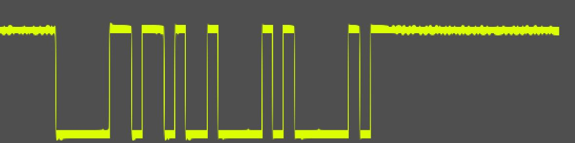
An actual depiction of a MIDI message as seen through an oscilloscope. MIDI speification determines two basic types of message bytes: the status byte and the data byte. The Most Significant Bit (MSB - or, first bit of a byte!) of a status byte is always 1. The MSB of a data byte is always 0. Lets first establish how a **status** byte works...
