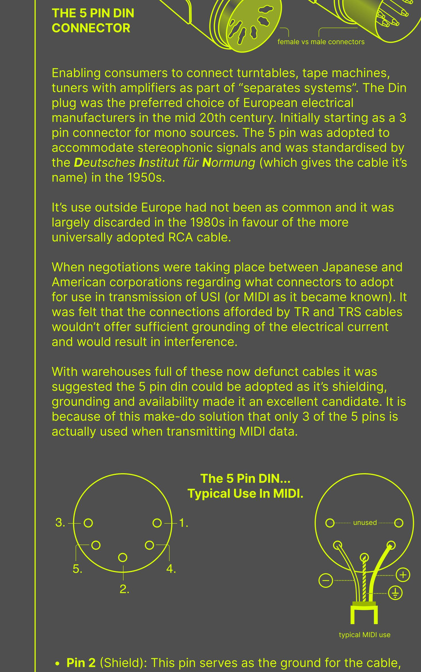
providing a return path for the signal and reducing noise. • Pin 4 (Current Source): This pin typically carries the positive MIDI signal. • Pin 5 (Current Sink): This pin typically carries the negative MIDI signal. • Pin 1 & Pin 3 (Unused): These pins are not used for standard MIDI communication, although they might be utilized by specific devices or applications.
