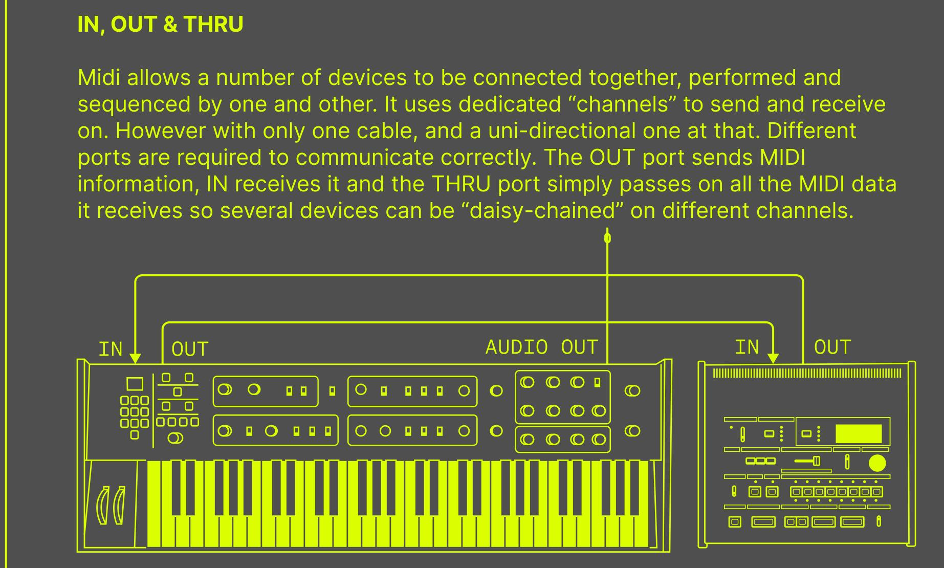
In this example the performer plays MIDI into the sequencer from a MIDI synthesizer to record. The sequencer then transmits the MIDI information back to the synthesizer to play back the performance from the sound being generated in the keyboard. The keyboard outputs that sound to a mixer, amplifier or pair of cans independently of the sequencer.
